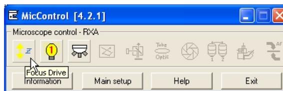
To access a particular feature of the microscope, click the corresponding tool. In the example above, the Z focus, lamp supply 1, and objective turret have been configured as available. To open the focus control dialog, click on the Focus Drive tool to display the corresponding dialog, as shown below. Similar dialogs are available for each component.
