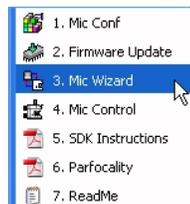
The Mic Wizard guides you through further detailed configuration of your microscope, such as specifying which objectives are fitted in each position on the nosepiece, defining the parfocality between lenses, and other options.
