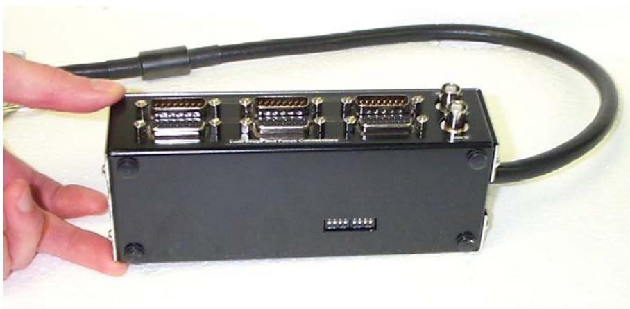
On the underside of the unit there are 8 DIP-switches which allow the selection of either rotary (via the motor connector), or linear (via the separate encoder connector) encoder type, for each axis, and
