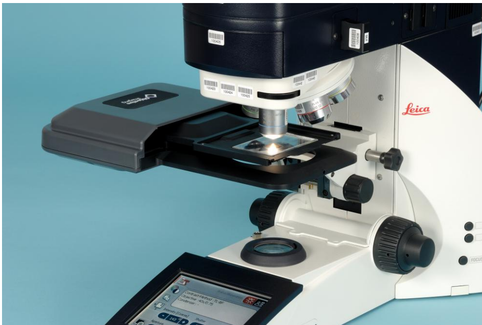
Figure 5. The Glide-S2 stage fitted to a Leica Microsystems DM6000 microscope. Note the side mounting of the electronics assembly (under the grey cover). The Glide is designed to allow mounting with the electronics to either the left or right sides. See the Appenices for mounting instructions.
