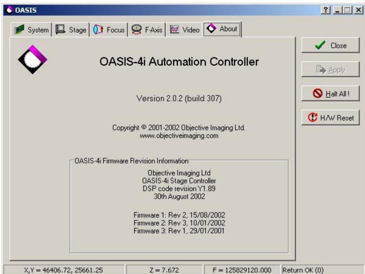
In the OASIS-4i Firmware Revision Information section, the DSP code revision should be Y1.89 or later, and Firmware 1 should be Revision 2 or later.
