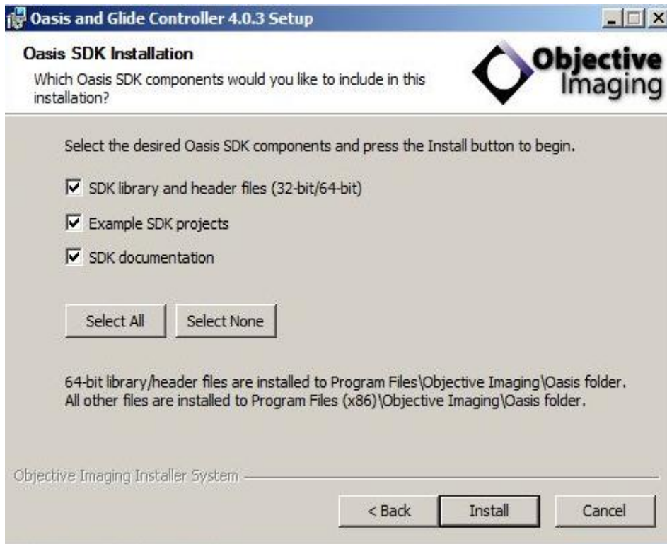
Figure 10. Oasis SDK Installation. This installs the interface files for software developers to incorporate the Glide into their applications.
